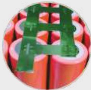
Laser Spot Welding on Li-ion Battery Tab
